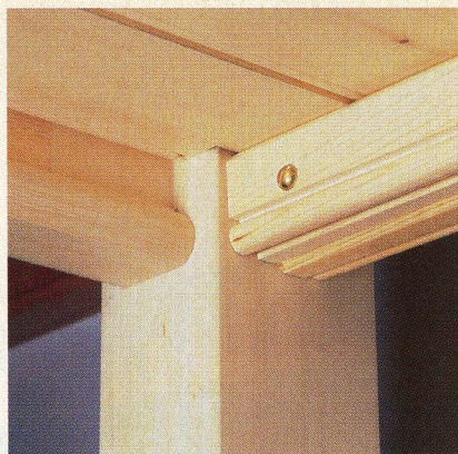
THE CORNER of the underside of the top bunk, showing mattress support boards, mattress support strip and the bottom of the headboard where it joins the leg
